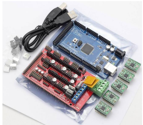
Fig 3.1: Arduino with motor drivers and ramps 1.4 shield [7].
