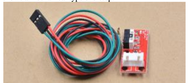
Fig 3.7: End stop (Mechanical switch type) [13].
